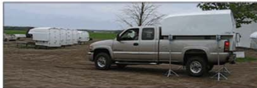
Camper style heavy duty "Jacks" capacity of 2000 pounds
