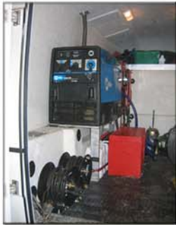
Repair unit with generator
